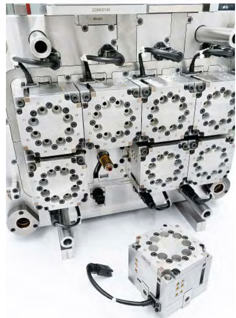
Tooling for the manufacture of pipette tips, with a double quick-change system. Each heating element can be removed individually in no time
