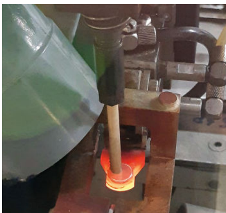
The copper inductor installed and tested
