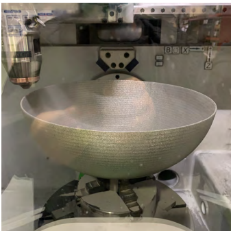
Satellite tank half shell production
