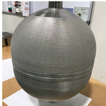
Satellite tank made out of Titanium
