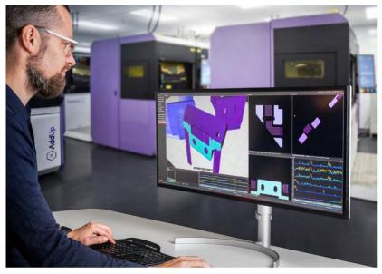
AM Explorer by Interspectral, displaying meltpool data from AddUp's FormUp 350 system.
