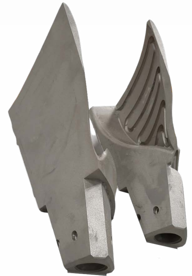
3D printed injection mold with AISI 420 steel
