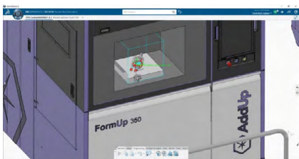
Virtual twin of FormUp 350 integrated in the 3DEXPERIENCE platform.
