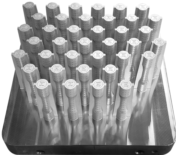
IN-718 fatigue specimens built on AddUp's FormUp 350 Powder Bed Fusion machine.
